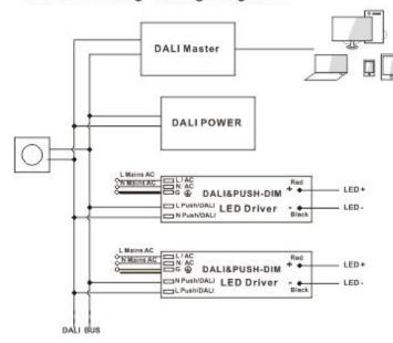
Push-Dimming Wiring Diagram1
