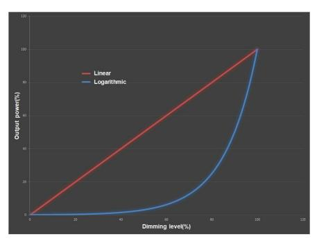
Note: Dimming curve: Logarithmic (default) and Linear
