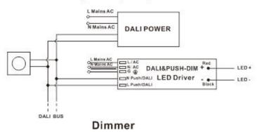
DALI Dimming Wiring Diagram2
