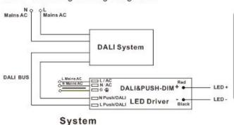
DALI Dimming Wiring Diagram3
