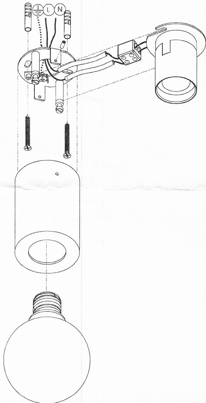
**General installation and maintenance directives concerning factory guarantee.** Connecting and testing the lamps must always happen by an acknowledged electrician according to the locally applying regulations on electric installations. Do not place on a flammable surface. All class I lamps must be earthed in the cable clamp marked with a  $\oplus$ -sign. Class II lamps may not be earthed. Disconnect from the main supply when fitting lamp or changing bulb.
